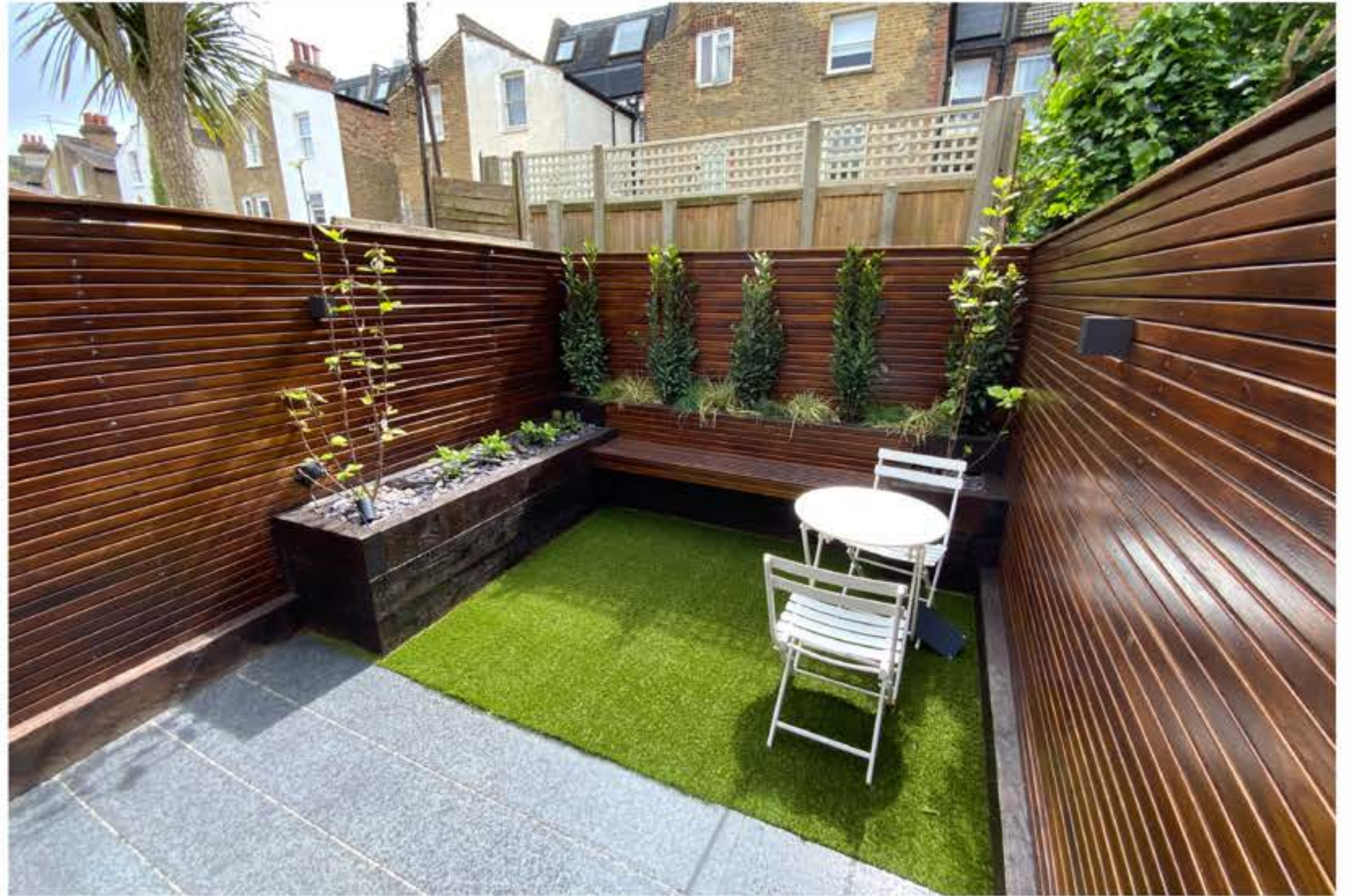
02 Softwood batten & sleepers used to create a budget friendly garden space.
